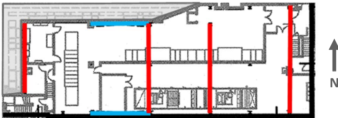
Figure 9 Floor plans showing braced (blue) and moment (red) frames locations in the central plant). (Courtesy of EwingCole)
