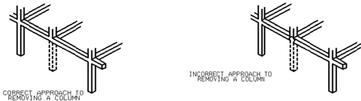
Figure 30 Images depicting the proper protocol required when removing a column for Alternative Path Analysis. (From UFC 4-023-03)
